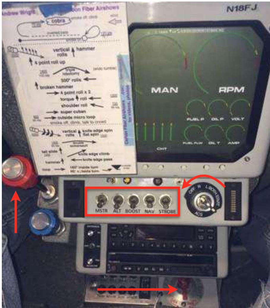
Pull the red mixture knob out to shut off fuel flow at the engine. To do this, you must press in on the center with your thumb while squeezing the red barrel. This will shut off a running engine.
