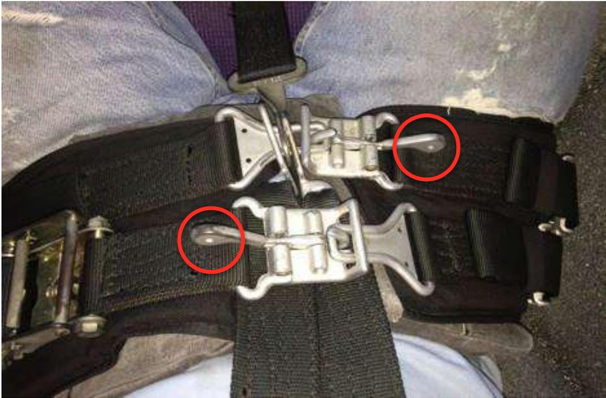
The pilot seat harness is released by pulling upwards on two levers as shown. The ratchet on the left side only tightens the belts, and will not aid in releasing them.
