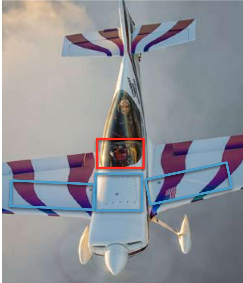
This aircraft has 3 fuel tanks, outlined in blue. The center tank, located in the fuselage, has a maximum capacity of 17 gallons. It will likely hold 5 to 12 gallons of 100LL during an airshow performance.
