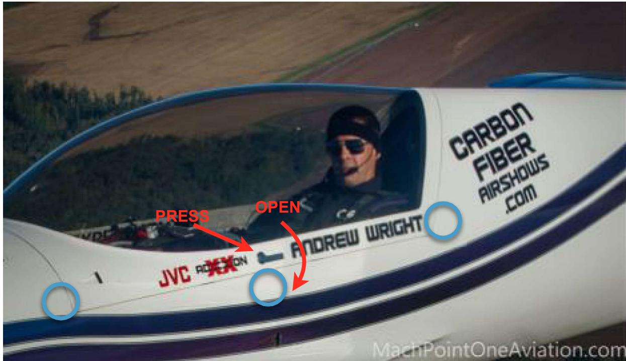
The external canopy release is a flat aluminum lever that sits flush in a recess in the middle of the left side of the canopy. Press in near the front of the lever to pop it out of the recess. Pivot the aft end of the lever down (clockwise) approximately 1/4 turn to disengage the latching mechanism. Then canopy then hinges open to the right.
