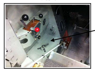
Fuel Selector Valve: Left side of front cockpit. Short end points to active position. Rotate 90 degrees clockwise to select "OFF".
