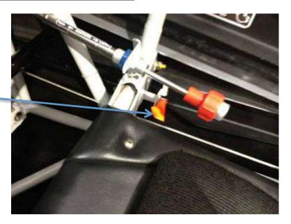
To shut off fuel: pull valve lever aft and rotate down to the 6 o'clock position.
