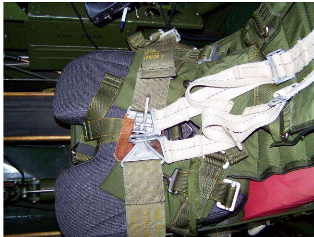
Military type harness – pull lever UP for Release
