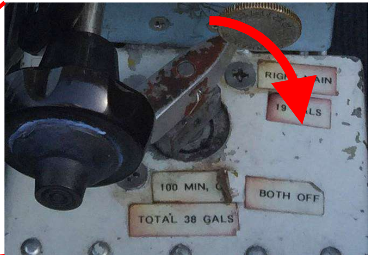
Rotate red valve at base of center console \frac{1}{4} to \frac{1}{2} turn COUNTER CLOCKWISE to the stop to shut of fuel supply.
