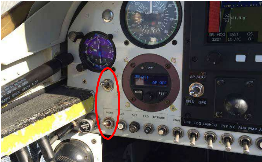
Two master switches control all electricity to the aircraft. DOWN is OFF.
