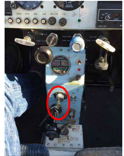
Engine ignition is killed by rotating the key on the center console COUNTER CLOCKWISE.
