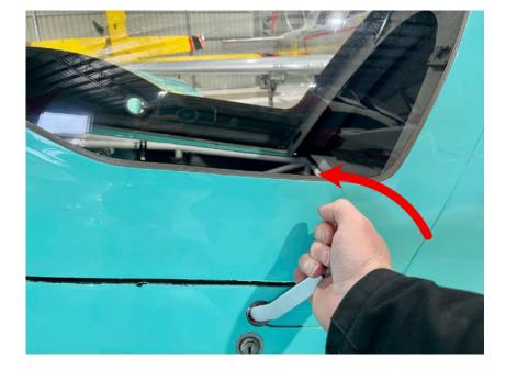
STEP 3 - LIFT canopy up and fold over to RIGHT
