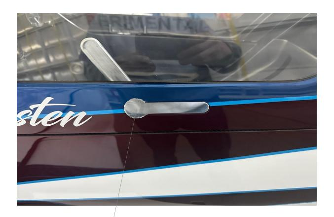
Upon Reaching aircraft push this lever in. Next Rotate it in a clockwise position to open the canopy. Once the canopy is open you can simply just push the canopy forward to come off its hinges.
