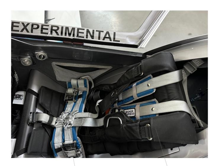
Next is to extract me from the aircraft. Simply pull on these levers. Undo the buckles, and place them off to the side.
