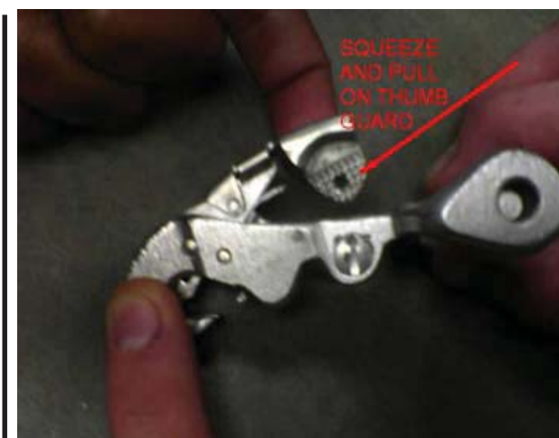
3g CHEST AND LEG STRAP EJECTOR SNAP WITH CATCH (PN 68D37721)
